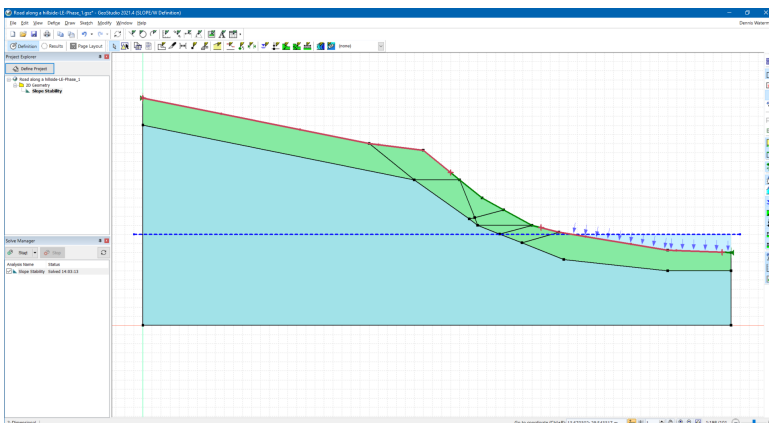
Figure 4.3: Model for Phase 1 in SLOPE/W
